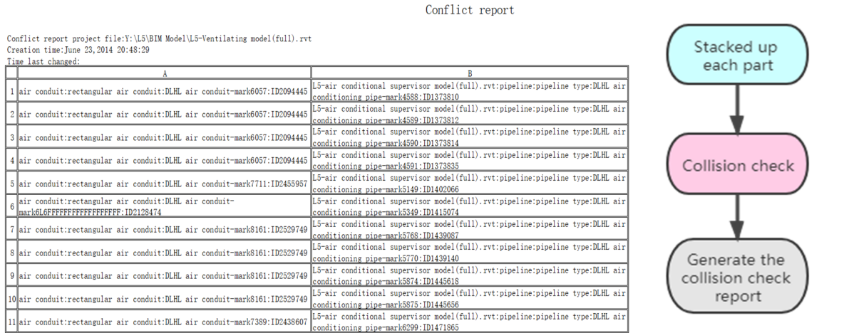
Figure 16 Pipeline collision detection
